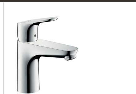
Focus - Single lever basin mixer 100 LowFlow 3.5 l/min without waste set
